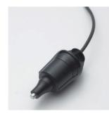
This reacts to the electromagnetic vibration, unaffected by the background noise. The measurement is possible under the vibration decrement early. However, an application such as the pasting of a thin magnetic film or the magnetic paint is necessary for a measurement side in the case of a rubber belt. (Entire arm length is 1m)
